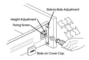
Tighten screws on Expanding Dowels.
