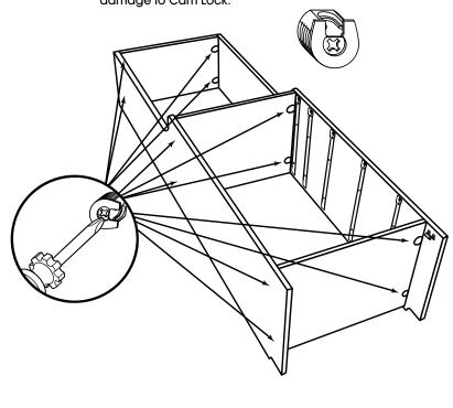
Attach Metal Plinth Catch vertically to Kickplate (H) using #6 x 1/2" Phillips Screw (Z) in center hole of catch. Then snap Kickplate into place.
