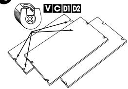
With Hutch Sides laying down on floor, assemble Fixed Shelves to Cam Bolts on Hutch Sides. **Note:** To lock into place, Cam Locks only require 20 lbs of force and a counterclockwise turn of 180 degrees. Excessive force or over tightening may result in improper assembly or damage to Cam Lock.
